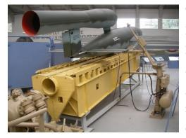
They were used in a campaign of "terror bombing" in British cities like London, in an effort to demoralize the British public. Their guidance system used a simple autopilot to control altitude and airspeed; a pair of gyroscopes controlled yaw and pitch; the azimuth was maintained using a magnetic compass; a barometric device was used to control altitude. The gyros, rudder,
